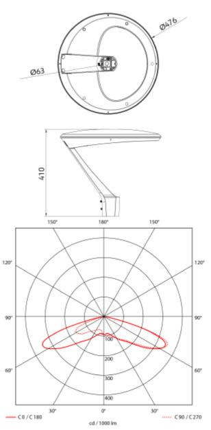
Modern and highly efficient post top luminaire for park and pathway. Theros Lite are IP66 and IK08 and available in 3000K or 4000K. Delivered with 5m cable, for Ø60mm mast.
