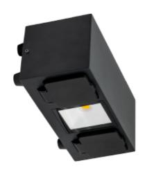
Outdoor luminaire with direct light and double outlet. Dimmable by phasecut. Easy installation with screwless terminal block. Made of powder coted aluminum. Included accessories: 4 spacer blocks for surface mounting
