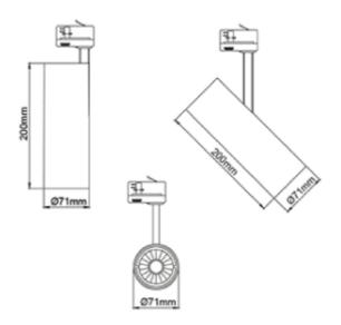
The Silindir uses the possibilities created by new technology. The LED driver is mounted inside the luminare body. This gives us a slim design combined with a powerful light output that can be easily adjusted in all directions to meet all needs. Cylinder can be tilted 90 degrees and rotated 350 degrees its own axis.
