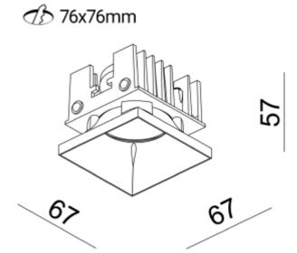
Square downlight suitable for most rooms. Single and double installation kit most be bought separately.
