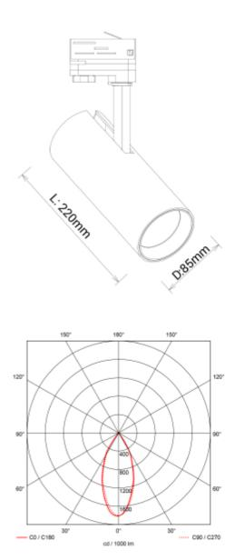
The Cylinder uses the possibilities created by new technology. The LED driver is mounted inside the luminare body. This gives us a slim design combined with a powerful light output that can be easily adjusted in all directions to meet all needs. Cylinder can be tilted 90 degrees and rotated 350 degrees its own axis. To create further opportunities to "play" with light you can mount a diffuser on the luminaire, this can be ordered separately.
