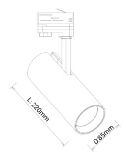
The Cylinder uses the possibilities created by new technology. The LED driver is mounted inside the luminare body. This gives us a slim design combined with a powerful light output that can be easily adjusted in all directions to meet all needs. Cylinder can be tilted 90 degrees and rotated 350 degrees its own axis. To create further opportunities to "play" with light you can mount a diffuser on the luminaire, this can be ordered separately.
