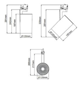
**(€** ☐ IP20 230V 50Hz **SPECIFICATIONS** Lightsource Type: LED (built in) System Power [W]: 39W CCT (Color Temperature): 4000K CRI / Ra: 90 Lumen LED (tc=25): 5200lm Beam Angle: 12° Lens (Diffuser): Clear Dimming: None System Voltage [V]: 230V 50Hz Connection: Track 3-Circuit Mounting: Ceiling MacAdam (SDCM): 3 Height [mm]: 281mm
