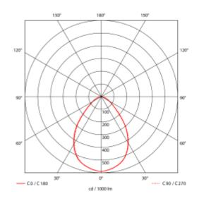
Antares downlight have high lumen output and PMMA diffuser with even light distribusion. Choose between opal or microprismatic diffuser. Comes with a switch option between 3000K(default), 4000K and 5700K. All data is based on 4000K.
