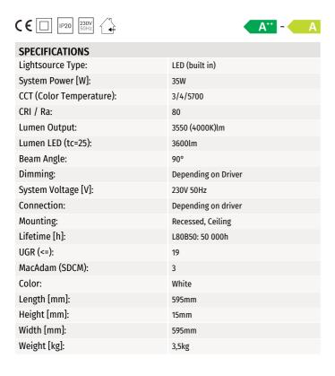
Panel Relax is a luminaire suitable for interior use. Ideal replacement for traditional 3x24W HO T5 and 3x18W T8 fluorescent louver luminaries and side lit LED panel light. Panel Relax have low glare and comfortable light. Comes with a switch option between 3000K(default), 4000K and 5700K. All data is based on 4000K.
