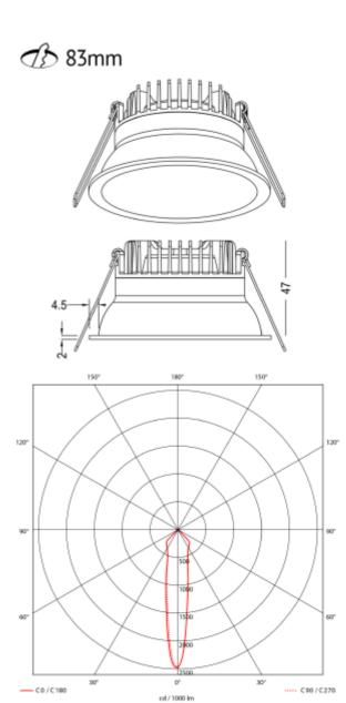
Ceto Mini fixed is a low downlight with 7W effect. With recessed light source, low blending, CRI95 and 18° beam angle, this is the natural choice where you want to create an exclusive and comfortable lighting. Phase-cut driver included.
