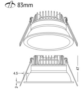
Ceto Mini fixed is a low downlight with 7W effect. With recessed light source, low blending, CRI95 and 18° beam angle, this is the natural choice where you want to create an exclusive and comfortable lighting. Phase-cut driver included.
