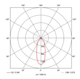
Ceto Mini fixed is a low downlight with 7W effect. With recessed light source, low blending, CRI95 and 36° beam angle, this is the natural choice where you want to create an exclusive and comfortable lighting. Phase-cut driver included.
