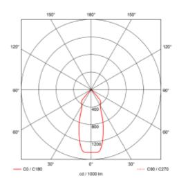
Ceto Fixed is a downlight with 15W effect and secluded light source. 36° beam angle and IP44 certified. Ceto Fixed is the natural choice if you are looking for an exclusive expression that provides a comfortable and good light. Dimmable phase-cut driver included.
