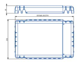
Adjustable downlightbox for recessed installation. With tape for easy installation. Length can be adjusted from 360mm to 570mm. Height 48mm. Holde size for 16 and 20mm tube.
