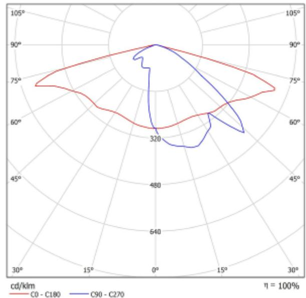
Anka is a luminaire for post mounting. We have developed this luminaire with an asymmetrical reflector giving a wide spread light, see light distribution diagram below. Anka has a post fixation opening with a diameter of 60mm. The luminaire has an IP66 classification and this guarantees that it will withstand very demanding conditions.
