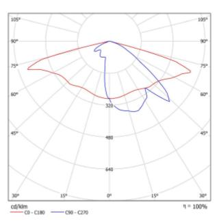
Anka is a luminaire for post mounting. We have developed this luminaire with an asymmetrical reflector giving a wide spread light, see light distribution diagram below. Anka has a post fixation opening with a diameter of 60mm. The luminaire has an IP66 classification and this guarantees that it will withstand very demanding conditions.
