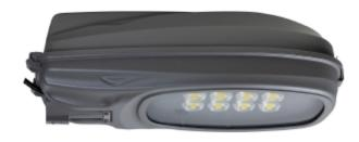
Aria is a LED luminaire for post mounting. We have developed this luminaire with an asymmetrical reflector giving beam angle of 60x120 degrees. Aria has a fixation of Ø60mm. The luminaire has an IP66 classification and this guarantees that it will withstand very demanding conditions. The Aria is available in several different models
