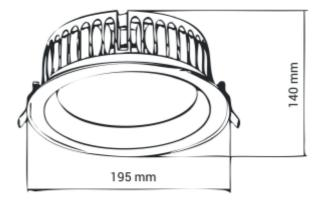
This series of IP44 downlights is named Auriga. Auriga is supplied with 2m cable for power connection.
