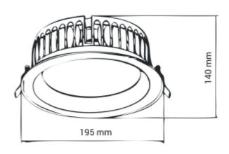
This series of IP44 downlights is named Auriga. Auriga is supplied with 2m cable for power connection.
