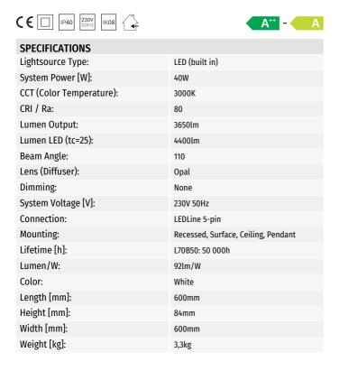
LEDline is a modern linear LED system for seamless lighting. It is based on modular chassis details allowing for seamless extensions through both straight connectors, 90 degrees corners and X-crosses. This allows light designers to make tailor fit lighting systems in an easy manner. The chassis details assure easy installation without failures. Add 1 pc 8050-05 for each mains supply (each row or standalone). Also add mounting accessories.
