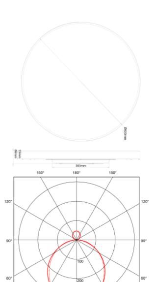
Galactic C is our new series of circular lamps. Modern design combined with prismatic diffuser that gives a pleasant and comfortable light. Galactic has several mounting options, recessed, semi-recessed, surface mounted or suspended. Choose between 2700K and 3000K (dip-switch) with direct light or direct / indirect light. Galactic is delivered in size: Ø400mm, Ø600mm, Ø800mm and 1000mm.
