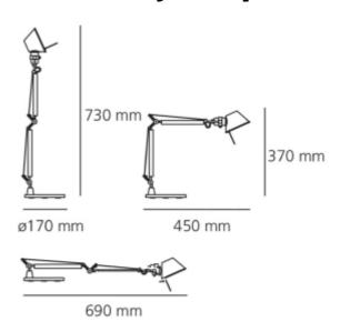
Base and cantilevered arms in polished aluminium; diffuser in matt anodised aluminium; joints and supports in polished aluminium. System of spring balancing.
