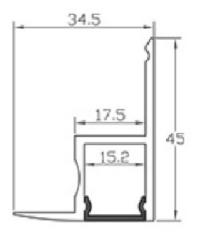
Aluminium profile for mounting on wall that becomes a part of the ceiling, and gives a decorative and modern light along the wall. Perfect where you wish to break up with a constant lighting line. Includes opal cover and end caps.
