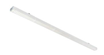
Trunk Line is our new fixture within technical lighting. This product is composed of two luminaires: Trunk with the optics of the T-line. Trunk Line is 50W, but the brightness can be adjusted down to 35W, 40W or 45W using the DIP switch on the driver. Supplied in 3000K with  $60^\circ$  light spread. Choose between on/off or DALI version. Power level with DIP switch:  $50W = 8500 \text{Im} \mid 45W = 7850 \text{Im} \mid 40W = 7100 \text{Im} \mid 35W = 6325 \text{Im}$
