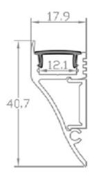
Aluminium profile for mounting on wall. Can be used as up or down lighting as indirectly lighting of ceilings, or as decorative lighting to highlight details. Cables can be hidden inside the profile. Includes opal cover, mounting clips, screws and end covers.
