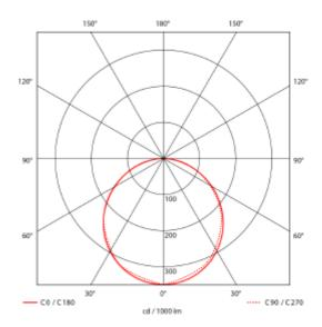
Panel LED is a light fixture for interior use. It is constructed for fitting in to suspended ceilings. Panel LEDs can be installed as a pendant or mounted on ceiling surfaces. The Panel LED has an opal or micro prismatic diffusor. Choose between ON/OFF, Phase-Cut or DAL12 (CLO, Corridor, Push dim and Ready2mains) driver. See accessories for detailed information.
