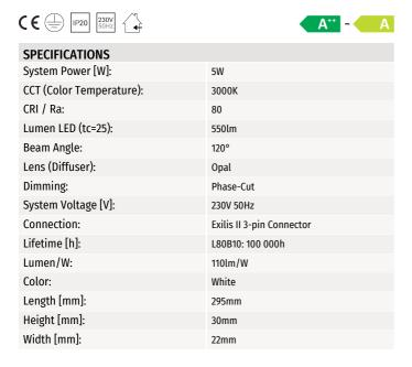
Our LED tube luminaire with a built in LED driver makes installation a breeze. The Exilis II comes in a variety of lengths that can be easily be connected together without the use of tools, just by clicking the LED tubes together. The different lengths makes it very easy to make a continuous line of light regardless of the length of the surface. The Exilis II comes with a opal diffuser and phasecut dim. Max 500W for each feed.
