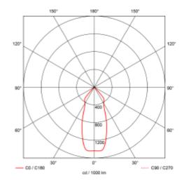
Ceto Fixed is a downlight with 15W effect and secluded light source. 36° beam angle and IP44 certified. Ceto Fixed is the natural choice if you are looking for an exclusive expression that provides a comfortable and good light. Dimmable phase-cut driver included.
