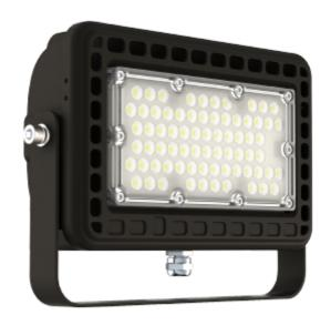
Colonel is a range of flood light fixtures mainly for outdoor use. The Colonel fixtures are made in robust die cast aluminum and are all IP66 classified. The fixtures are completely sealed and the vacuum inside prevents any condensation. The Colonel range is available in a number of models with wattage from 29W to 65W. The fixtures come with a mounting bracket and 50 cm power cord with an open end for easy installation.
