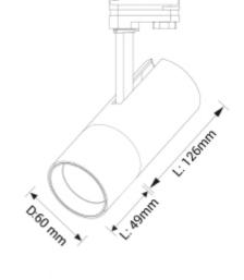
The Cylinder 60 has the LED driver included in the lamp head and is available for use in 1-circuit and 3-circuit tracks, both models are available with a Dim to Warm option. It can be tilted 90 degrees and rotated 350 degrees on its own axis and comes with a variety of accessories.
