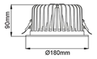
Leila C Midi is a highly efficient downlight with 126 lm/W. With wide beam angle and rotationally symmetric light distribution, it's suitable for all place that requires high lumen output. Can be delivered with on / off, phasecut or DALI2 driver. See accessories for suitable driver.
