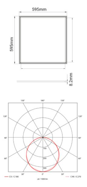
Panel LED is a light fixture for interior use. It is constructed for fitting in to suspended ceilings. Panel LEDs can be installed as a pendant or mounted on ceiling surfaces. The Panel LED has an opal or micro prismatic diffusor. Choose between ON/OFF, Phase-Cut or DALI2 (CLO, Corridor, Push dim and Ready2mains) driver. See accessories for detailed information.
