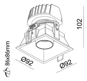
Make is a square downlight in singel version that comes with Dim 2 Warm function. The color temperature (K) can be adjusted between 3000K and 1900K through dimming. Rotatable 360° and tiltable 20°. Driver is not included and sold separately. See accessories for recommended drivers.
