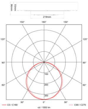
Galactic C is our new series of circular lamps. Modern design combined with prismatic diffuser that gives a pleasant and comfortable light. Galactic has several mounting options, recessed, semi-recessed, surface mounted or suspended. Choose between 2700K and 3000K (dip-switch) with dircet light or direct / indirect light. Galactic is delivered in size: Ø400mm, Ø600mm, Ø800mm and 1000mm.
