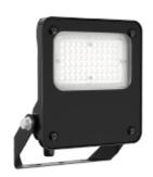
lota Marine is ideal for outdoor use and sports facilities that require durable lighting capable of withstanding challenging weather conditions. This LED light has a C5 corrosion class and IP66 rating, providing extra protection against water and dust. Additionally, lota Marine offers a lifespan of up to 100,000 hours (L80B10) and delivers flicker-free illumination
