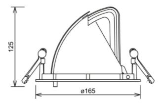
Zeta Mini is a small flexible LED downlight replacing the well-known Zebra mini, offering the same great quality and adjustment possibilities. The Zeta mini is supplied with 18i3 cable connector and can be delivered with a variety of connection options. The down light is available in three different colors.
