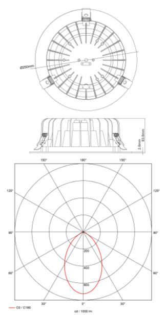
Leila R with cut out Ø210-240mm. Developed to change from halogen to downlight with latest LED technology. High Efficiency, easy installation. Delivered without driver. See accessories for correct driver-
