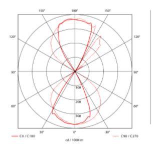
Matar has a unique feature were you separately may adjust the up and downward beam angle. This will allow the planner to fix the perfect beam angle for a diversity of applications. A timeless and slim design makes Matar the perfect choice for a glare free fasade light, suitable both for home or decorative commercial use. Integrated slides allows for adjusting the two beam angles from 0°-90°. Body in cast aluminium, with clear diffusers, and color in Dark Grey.
