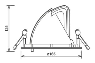
Zeta Mini is a small flexible LED downlight replacing the well-known Zebra mini, offering the same great quality and adjustment possibilities. The Zeta mini is supplied with 18i3 cable connector and can be delivered with a variety of connection options. The down light is available in three different colors.
