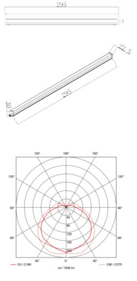
Our LED tube luminaire with a built in LED driver makes installation a breeze. The Exilis II comes in a variety of lengths that can be easily be connected together without the use of tools, just by clicking the LED tubes together. The different lengths makes it very easy to make a continuous line of light regardless of the length of the surface. The Exilis II comes with a opal diffuser and phasecut dim. Max 500W for each feed.
