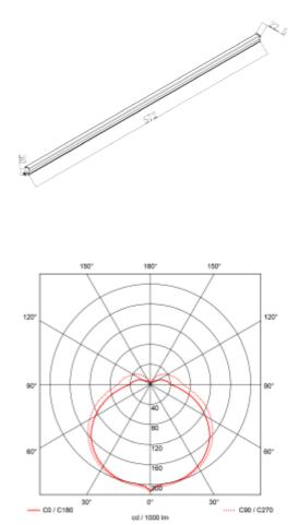
Our LED tube luminaire with a built in LED driver makes installation a breeze. The Exilis II comes in a variety of lengths that can be easily be connected together without the use of tools, just by clicking the LED tubes together. The different lengths makes it very easy to make a continuous line of light regardless of the length of the surface. The Exilis II comes with a opal diffuser and phasecut dim. Max 500W for each feed.
