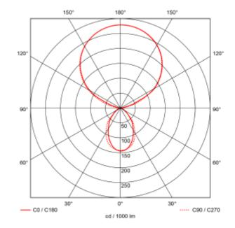
Benu is a linear LED luminaire with up- and down light for pending down in indoor areas. UGR<19 and dimmable by pulling the rope. 18i3 connection, 3000mm wire and t-profile bracket are included.
