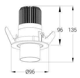
Zoom Recessed, is relatively small downlight with a cut-out size of Ø81mm. The unique zoom patent makes it possible to vary the beam angel between 5 - and 60 degrees making this model highly versatile. The Zoom Recessed is available in both 2700 and 3000 Kelvin and is made from robust die-cast aluminum. Please see the table for technical details.
