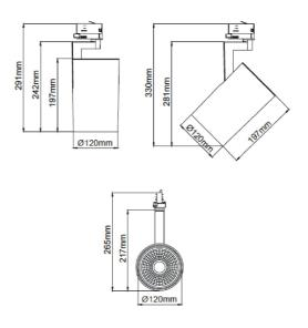
Ray Maxi, a powerful spotlight in the Ray family using a design concept with the LED driver built in to the spotlight body. This gives a modern, slim design with a high lumen output. The Ray Maxi can be tilted 90 degrees and rotated 350 degrees on its own axis offering create flexibility in playing with light. A diffuser can be mounted on the luminaire, to be ordered separately.
