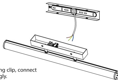
Remove the line pressing clip, connect the wires correspondingly.
