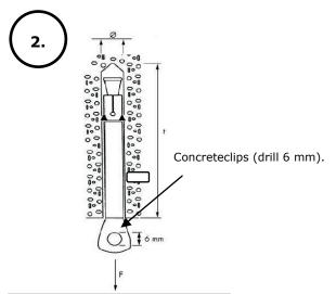
NOTE! Make sure the ceiling attachment can handle installed load with 5-fold safety.
