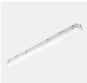
Duna is a sealed industrial light fixture for ceiling surface mounting, indoor or outdoor under a roof. Duna may have 5x2,5mm2 PG through-wiring. Opal PC (IK08) or PMMA (IK03) diffusor. Ask for Chemical agents list to check material resistance. Available models can be delivered with master (sensor), slave, DALI or emergency.
