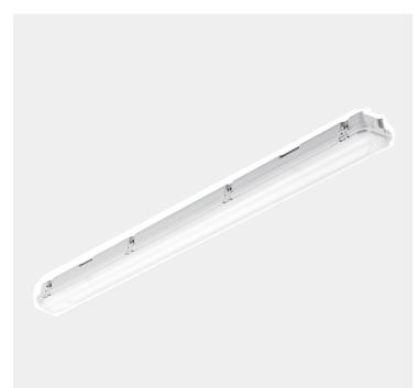
Duna is a sealed industrial light fixture for ceiling surface mounting, indoor or outdoor under a roof. Duna is classified in accordance with IP66 / IK08. The light fixture is made from robust fiberglass and is equipped with a semi-opal PC diffuser. 5x2,5mm2 PG through-wiring. Can be used together with 10184745 as slave luminaire (5pcs can be connected to one master).
