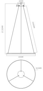
The Halo pendant range consists of 3 different sizes circular luminaires, they are made from aluminum, coated with a golden matt color. The opal surface covering the LEDs gives a very pleasant warm light in 3000 Kelvin. The length of the wires holding the circular luminaires can be adjusted on site making the Halo pendant very flexible for decorative purposes (wire length: 200cm).
