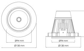
This is by far our most popular mini" downlight and it offers huge flexibility, tiltable up to 25 degrees. This downlight has a recessed light source giving a minimum of stray light. The Torres Mini can be supplied with a variety of connector solutions
